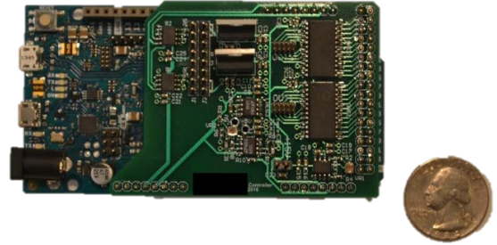
Figure 11—MoVR mirror’s controller board: The figure shows our custom-designed controller board for configuring the beam alignment and the amplifier gain in real time.
