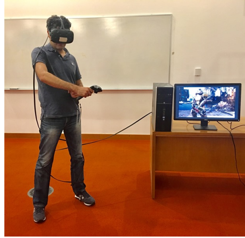
Figure 1—Virtual Reality experience: The figure shows the headset’s cable not only limits the player’s mobility but also creates a tripping hazard.
